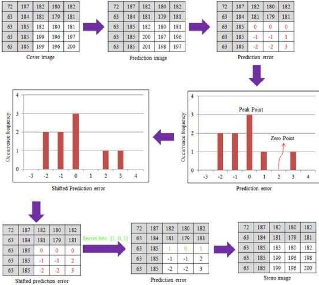
FIGURE 5. Example of embedding data using the proposed method
