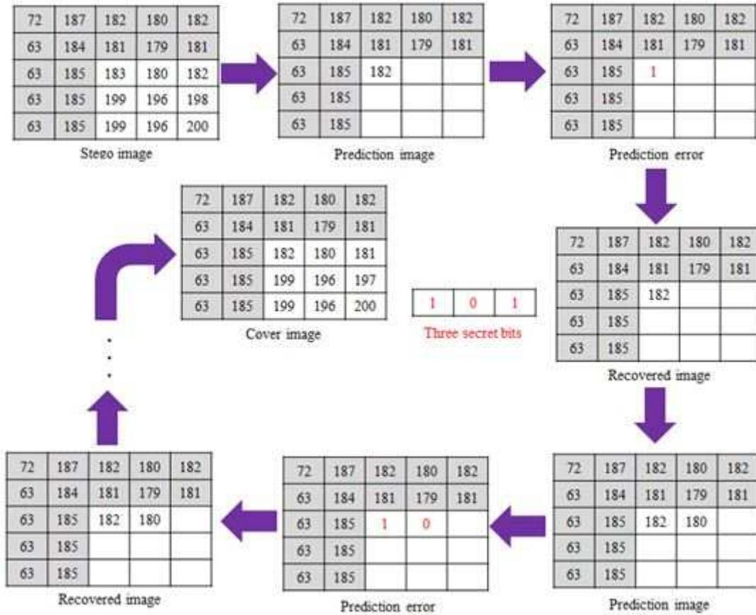
FIGURE 6. Example of data extraction and image recovery using the proposed method
