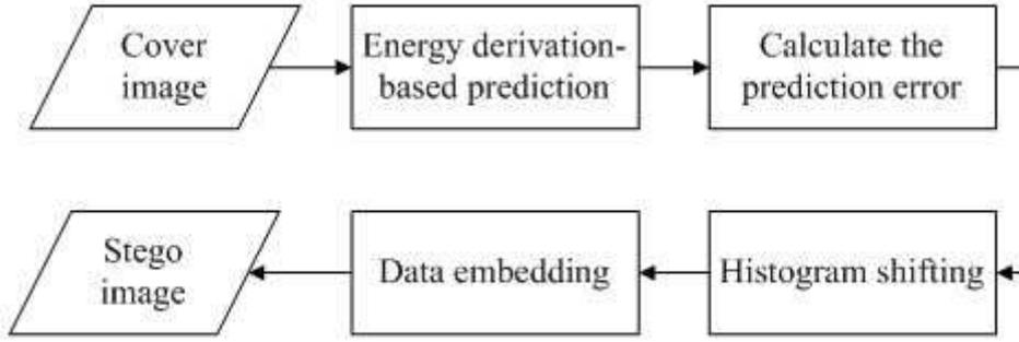
FIGURE 3. Flowchart of data embedding in the proposed method
