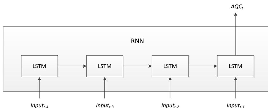
FIGURE 1. The process flow of RNN model for AQC forecasting
