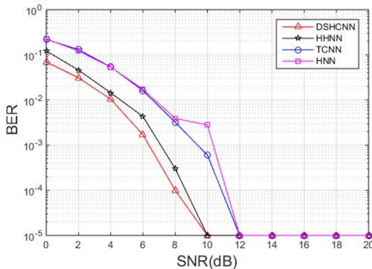
FIGURE 5. BER under random synthesis channel.
