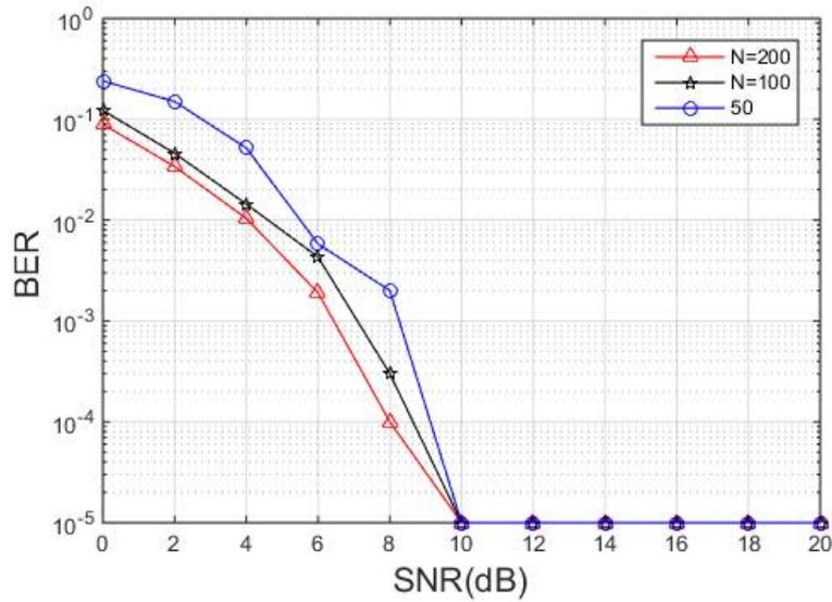
FIGURE 6. BER of DSHCHNN under different data.
