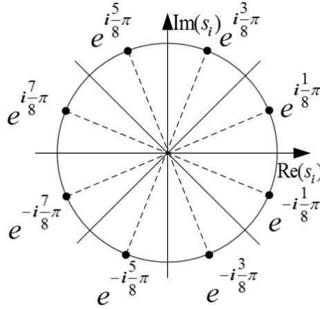
FIGURE 1. 8PSK signal constellation distribution
