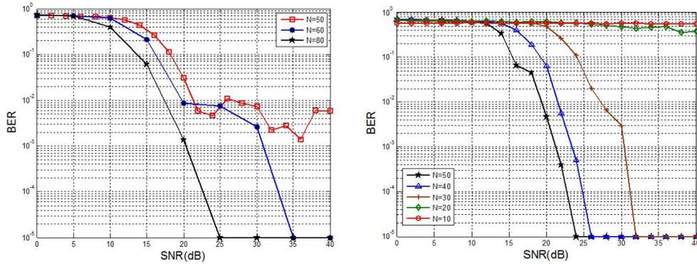
(a) CHNN-APHM algorithm with different data length (b) CTCNN-APHM algorithm with different data length
