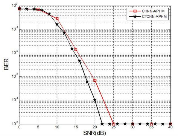
FIGURE 4. CHNN-APHM algorithm and CTCNN-APHM algorithm under random channel
