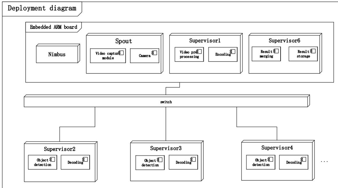
FIGURE 3. The intelligent target recognition front-end application architecture
