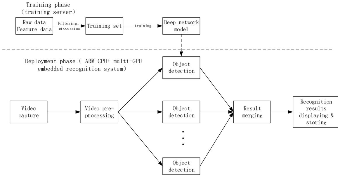
FIGURE 2. The overall process of target recognition
