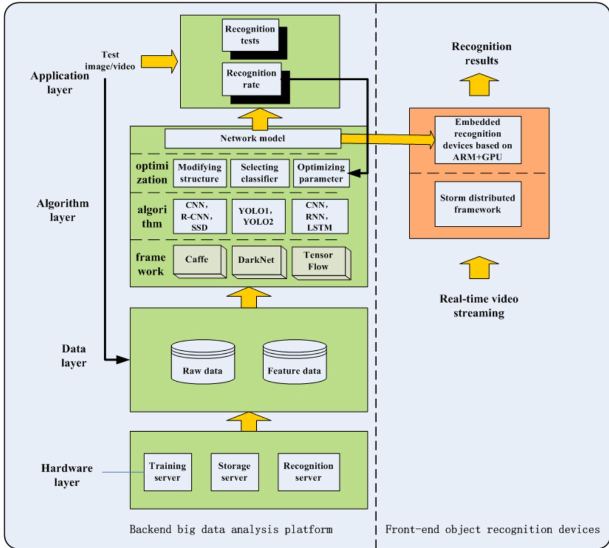
FIGURE 1. Architecture of deep-learning-based target recognition using high performance computing platform and embedded computing platform
