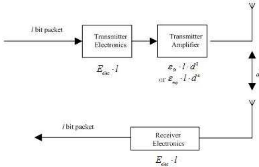
FIGURE 1. The radio energy consumption model
