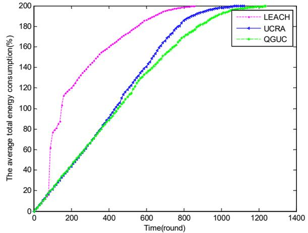
FIGURE 9. The average total energy consumption in LEACH, UCRA, and QGUC algorithm
