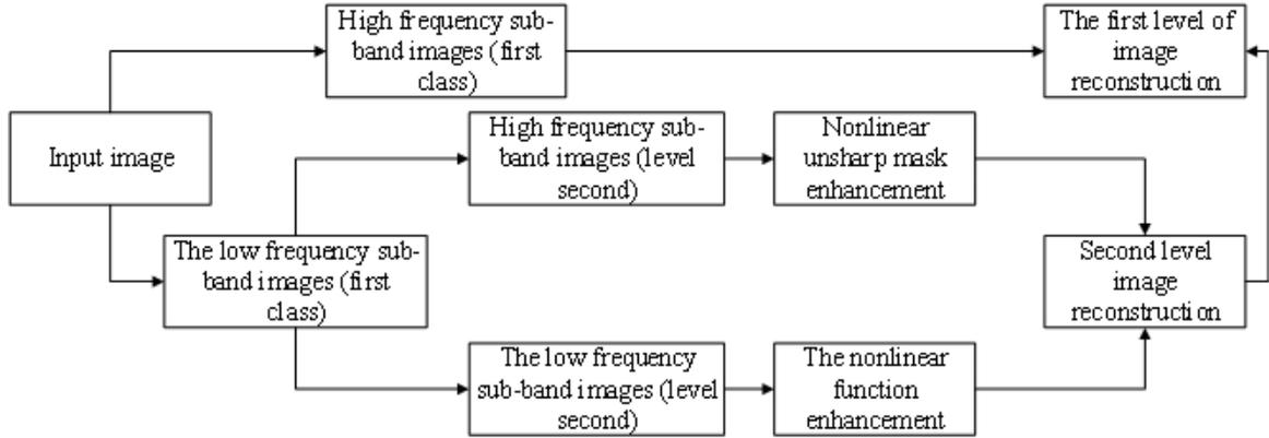
FIGURE 2. Flow chart of processing luminance component.
