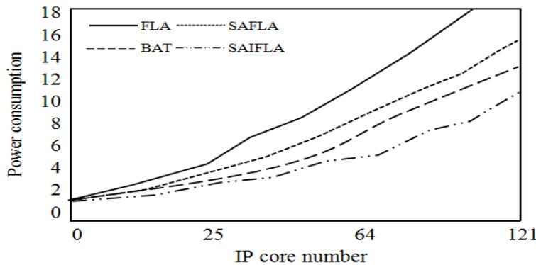
FIGURE 2. Power consumption comparison with increase of NoC size.
