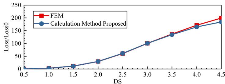
FIGURE 10. Comparison of Winding Losses by Analytic Method Improved and FEM
