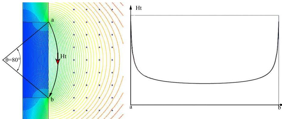
FIGURE 2. Flux lines around air gap (left) and field strength along line a-b (right)
