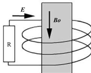
FIGURE 8. Equivalent Circuit of Proximity Effect
