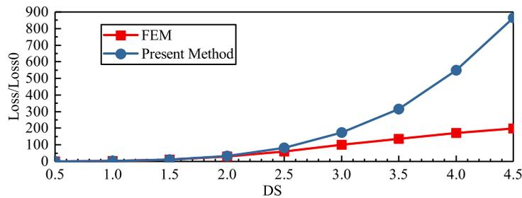
FIGURE 7. Comparison of winding loss by analytic method and FEM
