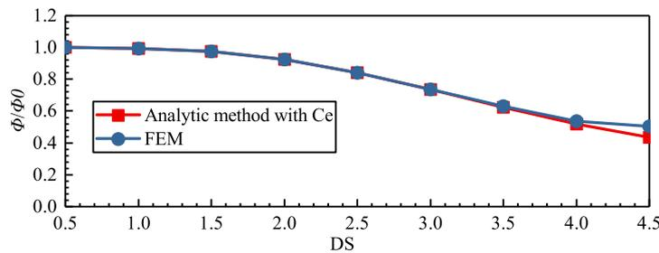
FIGURE 9. Comparison of the flux (a-b) calculated by analytic method proposed and FEM
