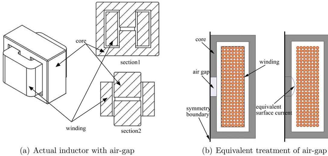
FIGURE 1. Actual inductor model and its 2D half model
