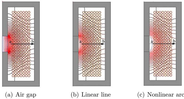
FIGURE 3. Flux lines distribution in winding window with air gap and different surface currents
