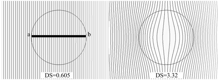
FIGURE 6. Flux line distribution in wire under different frequency
