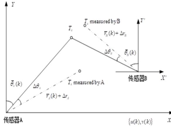
FIGURE 3. The geometric relationship of registration error.
