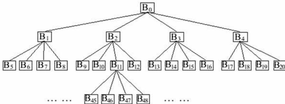
FIGURE 2. The Quaternary Tree Block Decomposition
