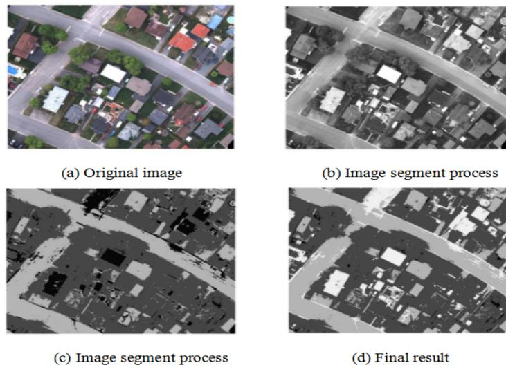
FIGURE 2. Fuzzy c-means clustering segment results.
