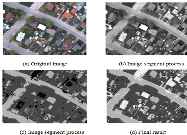
FIGURE 2. Fuzzy c-means clustering segment results.
