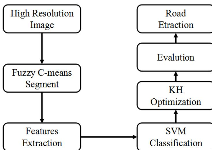
FIGURE 1. Framework of proposed road extraction method.
