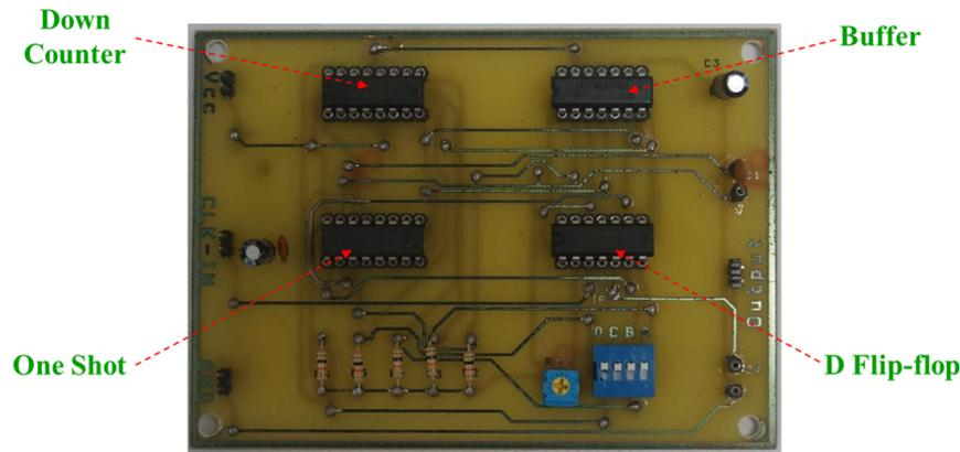
FIGURE 5. Circuit prototype of the proposed 4-bit DPWM
