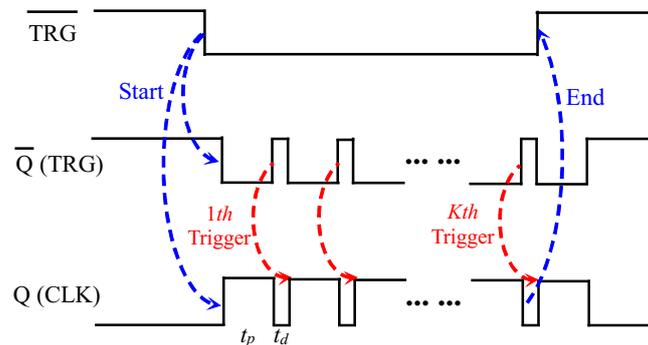
FIGURE 4. Self-trigger operation of one shot
