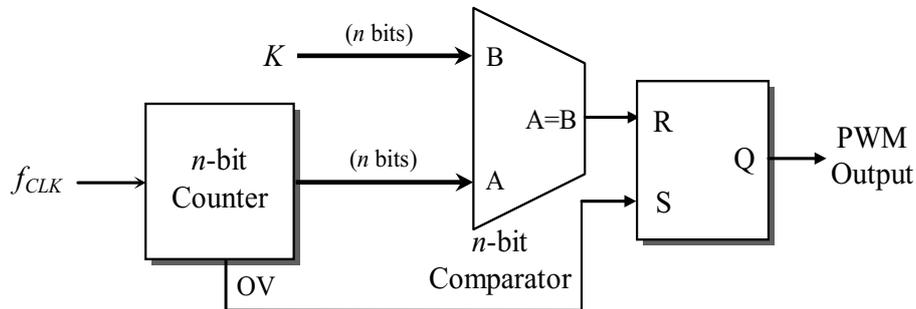
FIGURE 1. Basic structure of a counter-based DPWM
