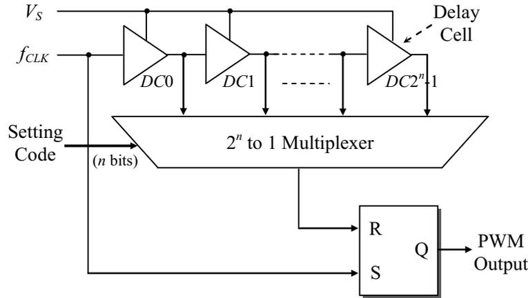
FIGURE 2. Basic structure of a delay-line DPWM
