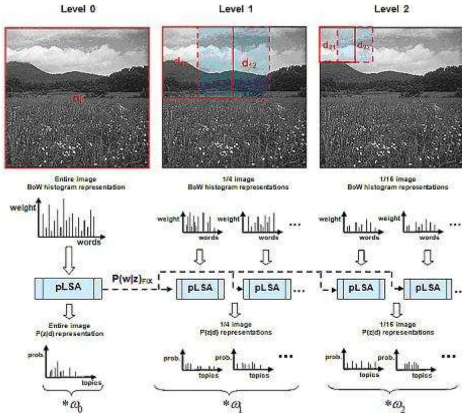
FIGURE 8. The structure of the cascaded PLSA model
