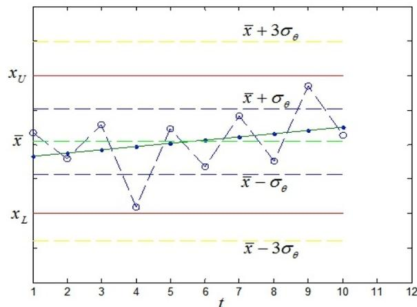
FIGURE 1. Schematic illustration of testing data for equipment performance parameter and its statistical characteristics
