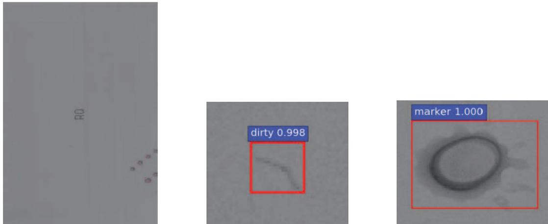
FIGURE 3. Example of the results of detecting defects in the image of the polarizer
