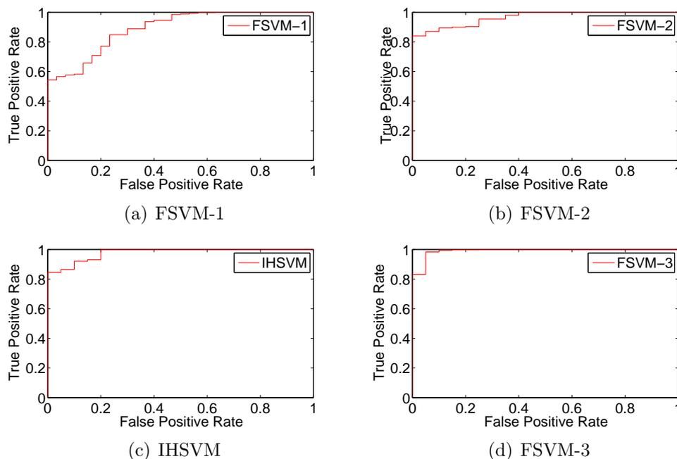
FIGURE 1. ROC curve of each model
