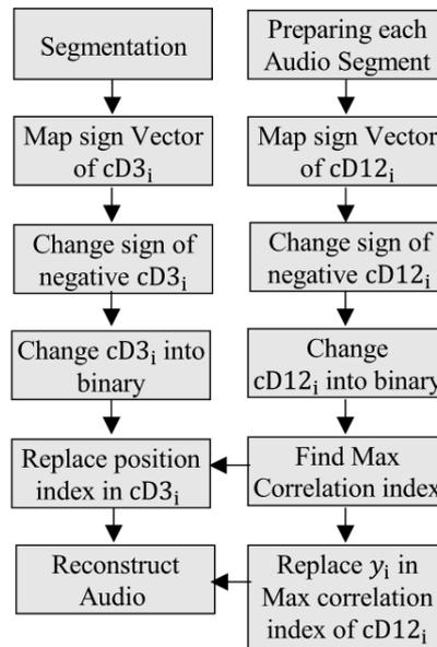
FIGURE 4. Bits Embedding location selection and Bits Embedding
