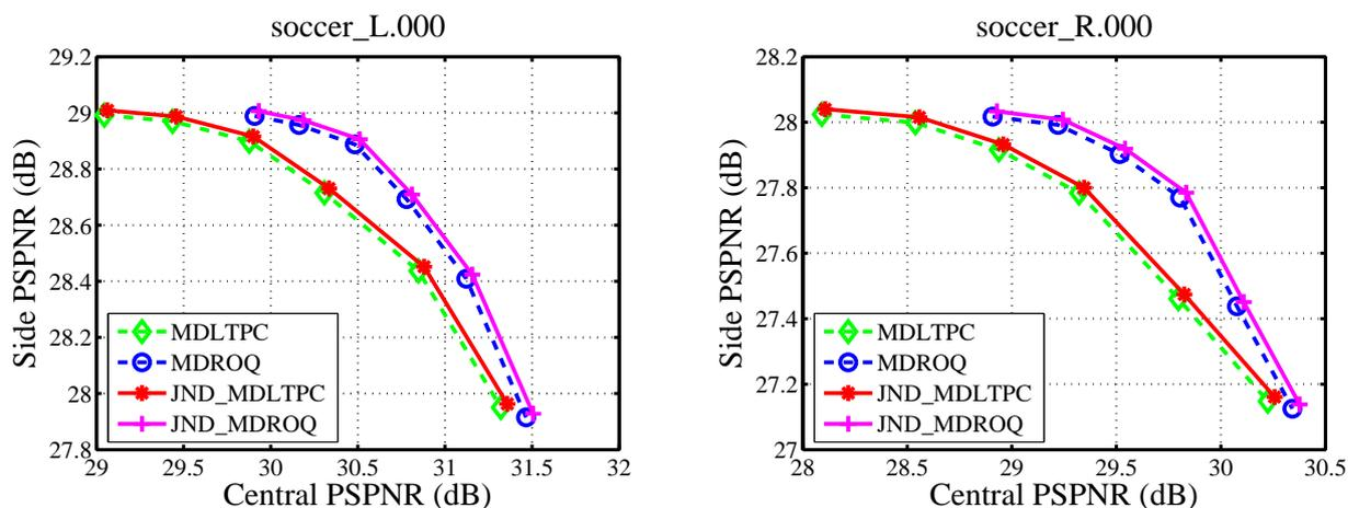
FIGURE 5. The side PSPNR vs. central PSPNR of various methods for Soccer and total rate of 0.5 bpp
