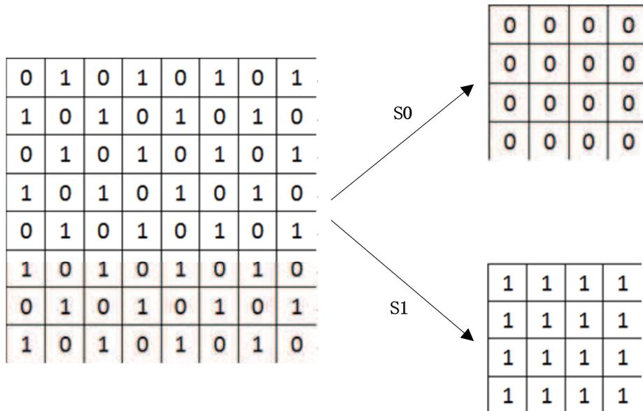
FIGURE 1. The block subset definition in 2-description image coding.
