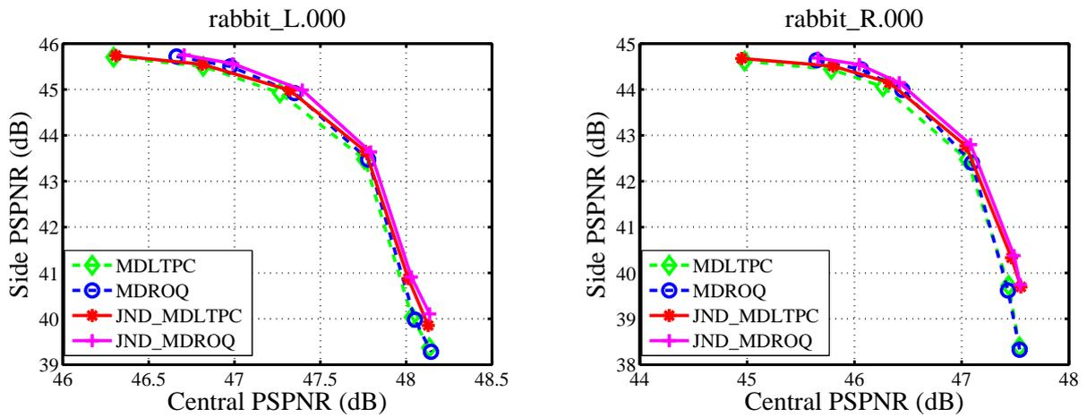
FIGURE 4. The side PSPNR vs. central PSPNR of various methods for Rabbit and total rate of 0.2 bpp
