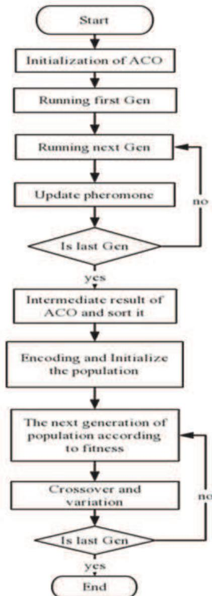
FIGURE 4. Flow Diagram of Our Proposed Algorithm
