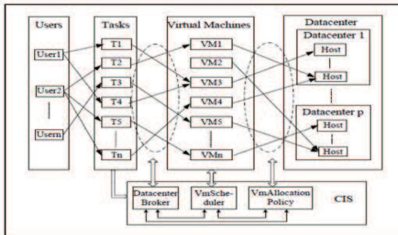
FIGURE 2. CloudSim Working Process
