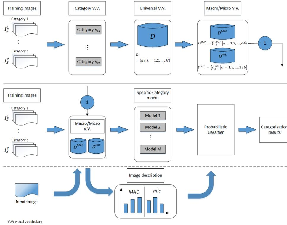
FIGURE 2. The structure of proposed image categorization
