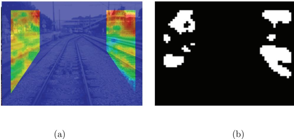
FIGURE 3. Example of saliency score and salient regions. (a) Heat-map of saliency score in ROI. The pixels with higher saliency score are drawn in red, while blue areas have lower saliency score. (b) The extracted salient regions.
