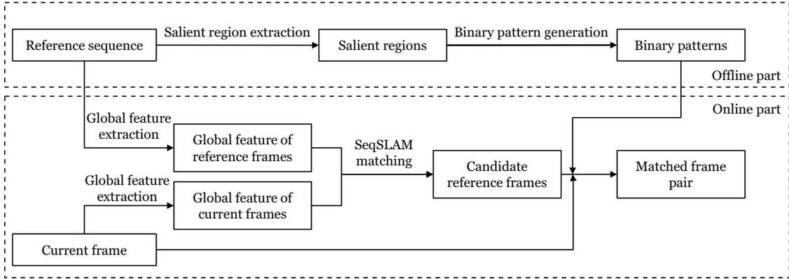
FIGURE 2. The framework of the proposed method
