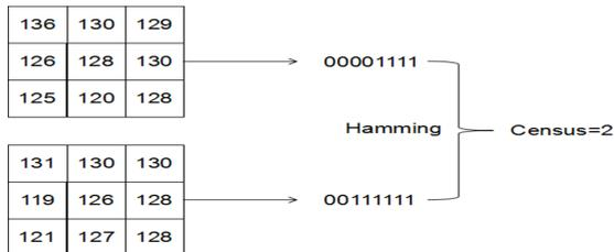
FIGURE 1. Census Transform schematic diagram
