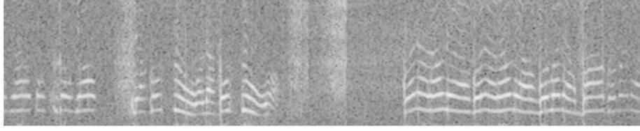
FIGURE 5. Non-Morse signal waveform
