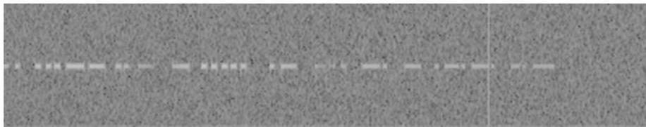
FIGURE 4. Morse signal waveform
