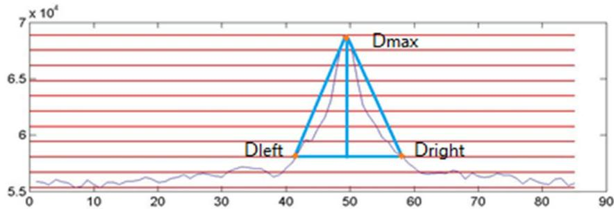
FIGURE 2. Symmetry level of Morse signal energy distribution
