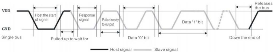
FIGURE 4. Data timing diagram
