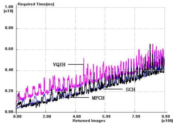
FIGURE 4. Comparisons of the feature extraction time needed for SCH, VQIH and MFCH for the database with 1000 images
