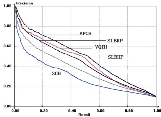
FIGURE 3. Comparisons of the average P-R curves among SCH, VQIH, SLBHP, SLBKP and MFCH with the same dimension of 192
