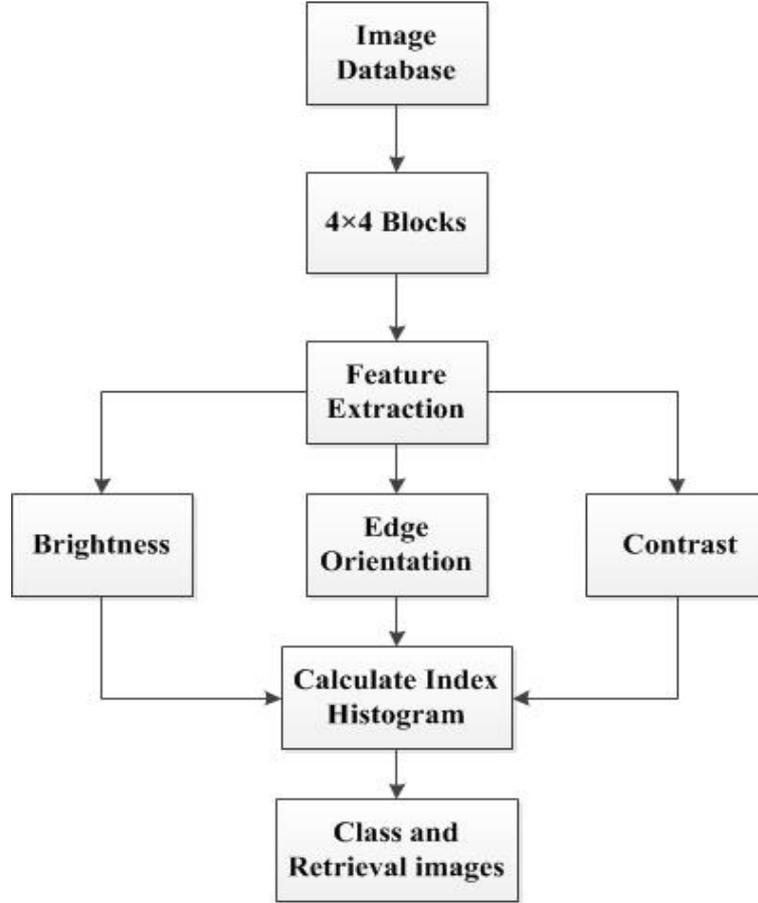
FIGURE 1. The feature extraction diagram of proposed algorithm
