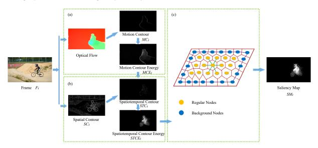
FIGURE 1. Illustration of the proposed framework. We integrate a new spatiotemporal contour energy in a graph model to cluster the salient object.
