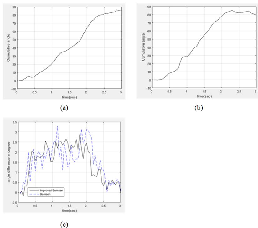
FIGURE 7. Results of angle measurement: (a)-(b) two curves of cumulative slope angle difference by Bernsen and improved Bernsen respectively (c) two curves of slope angle difference by two methods
