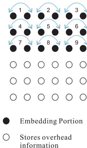
FIGURE 1. Illustrative example of pixel grouping when block size is  $6 \times 6$
