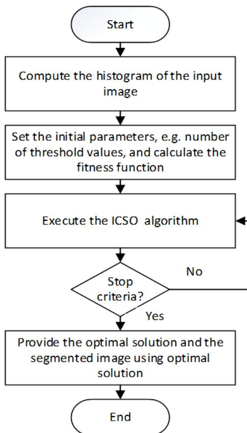
FIGURE 1. Flowchart of the multilevel image features extraction solution by applying the ISCO
