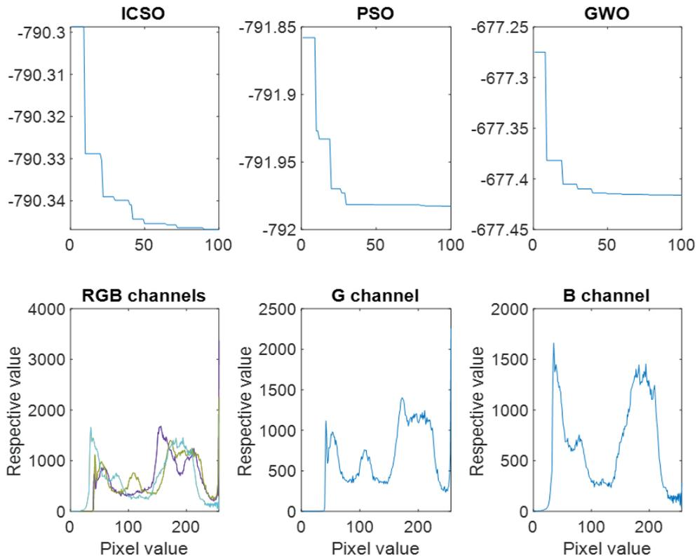
FIGURE 3. Comparison convergence of the proposed ICSSO scheme with the PSO [27] and GWO [23] methods and the visually extracted three channels (RGB) for image 1
