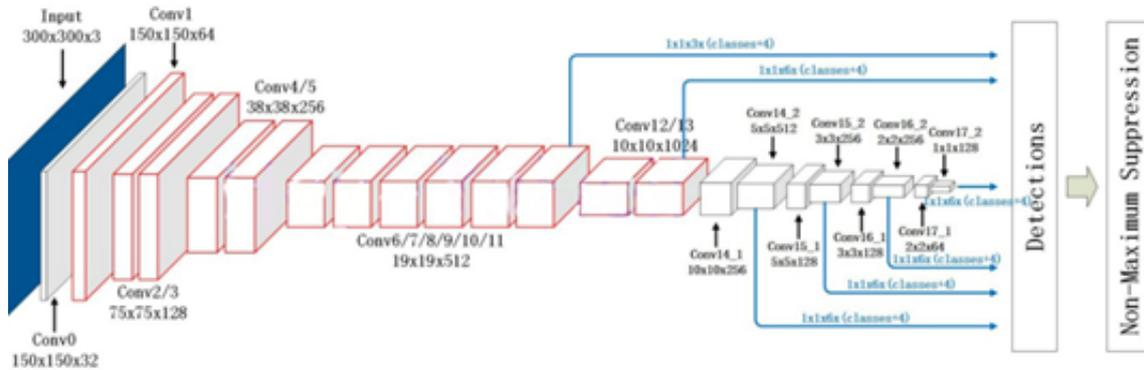
FIGURE 1. Structure of MobileNet-SSD
