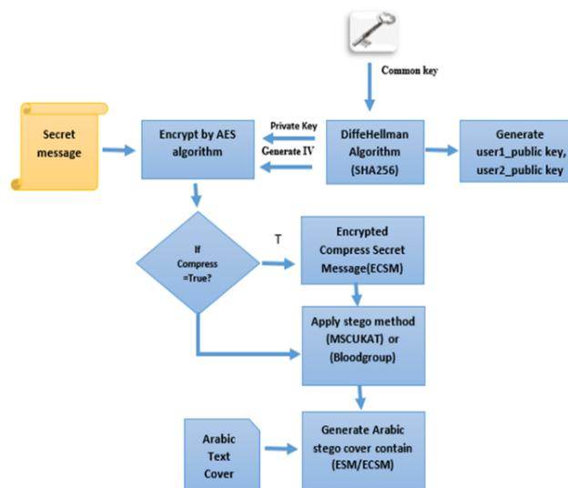
FIGURE 4. Encryption/Encoding Scheme
