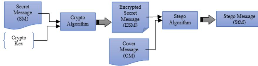
FIGURE 3. Typical crypto-stego method scheme
