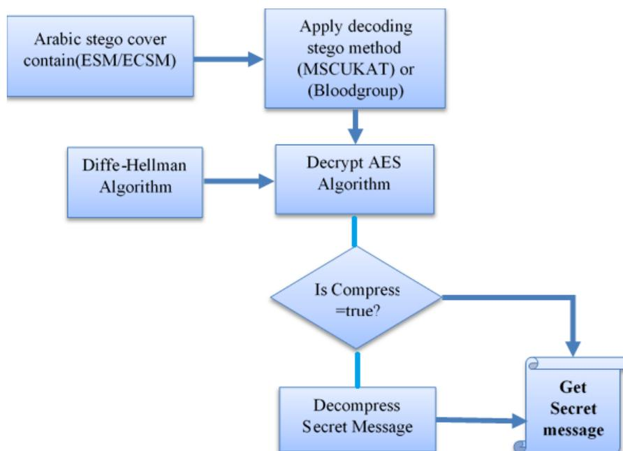
FIGURE 5. Decoding/Decryption Scheme
