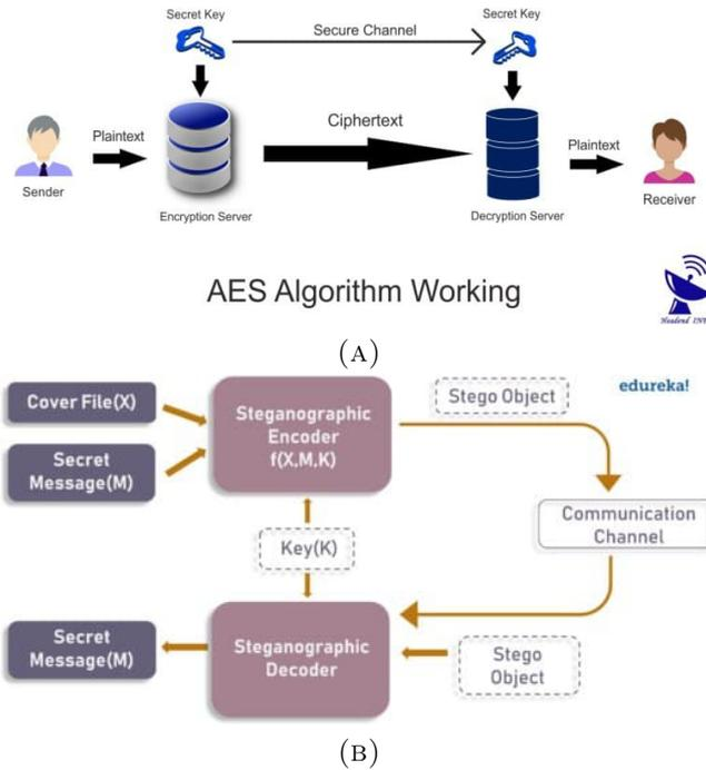
FIGURE 1. Standard security structure for, (a) Cryptography by AES algorithm [3], (b) Steganography [4].
