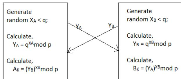
FIGURE 2. The algorithm of Diffie-Hellman key exchange [10].
