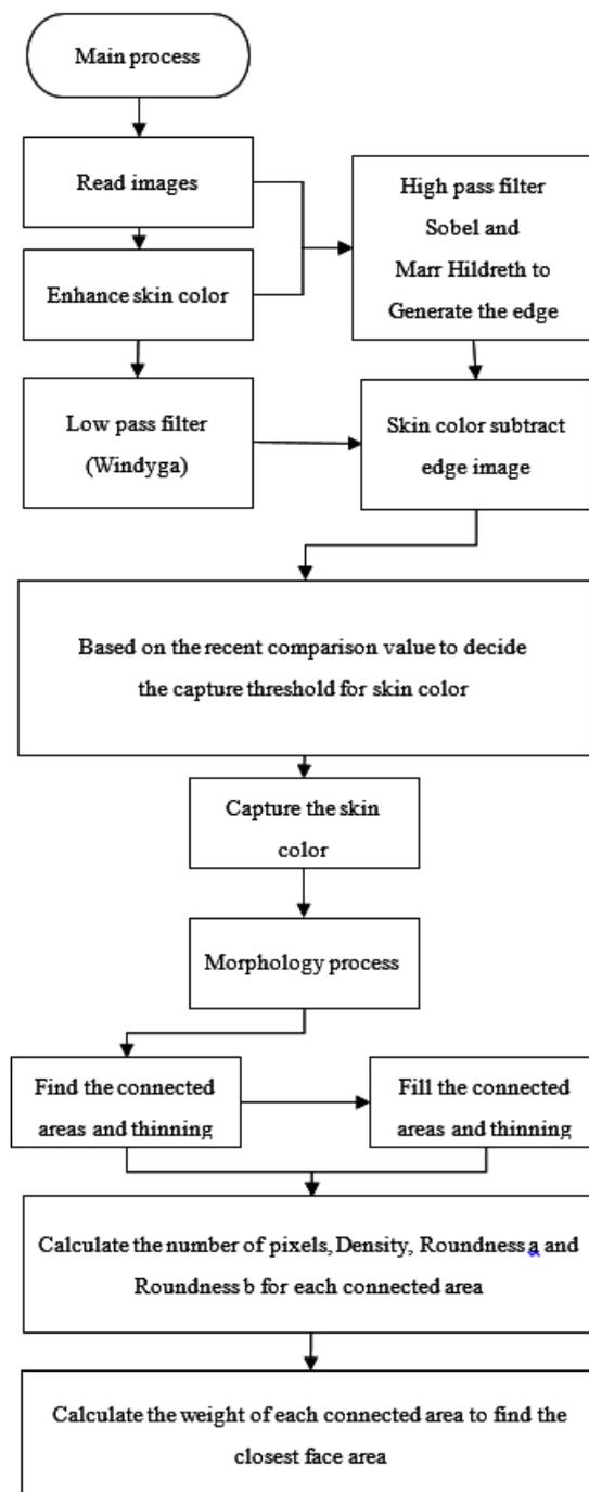
FIGURE 1. The static human face detection algorithm
