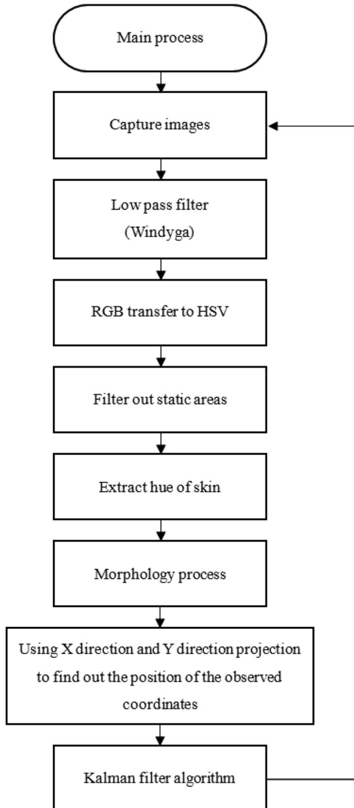
FIGURE 4. The flow diagram of dynamic face detection
