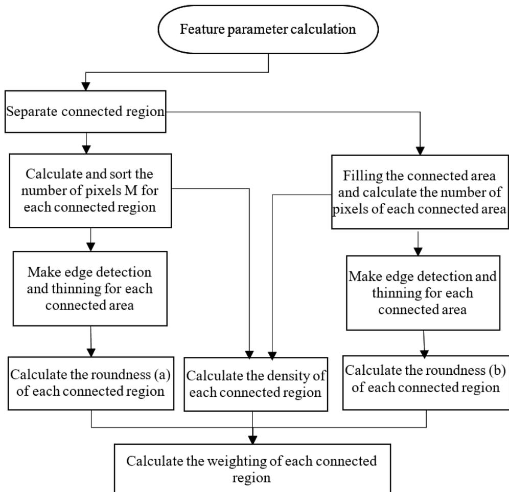
FIGURE 3. The calculation process of feature parameters and weighting
