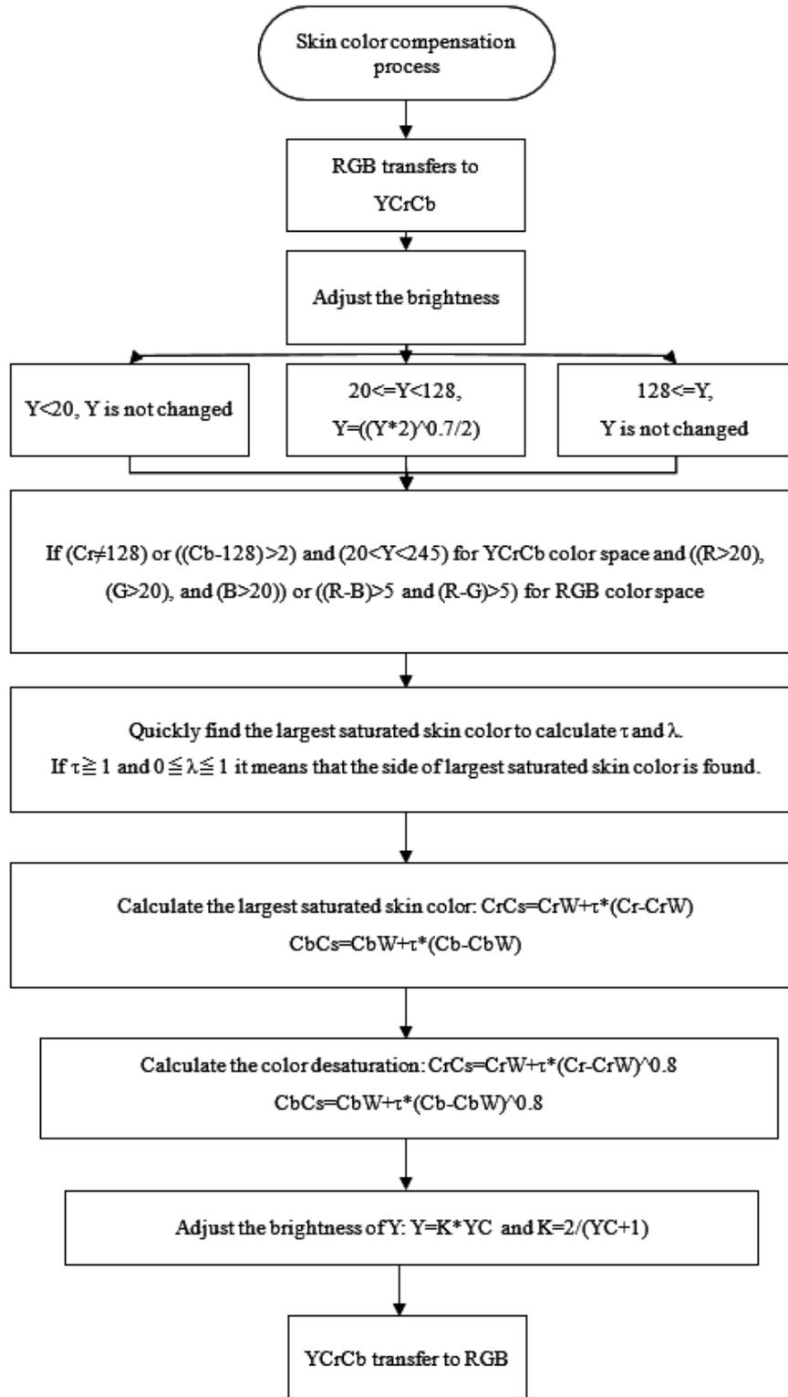
FIGURE 2. The color compensation process
