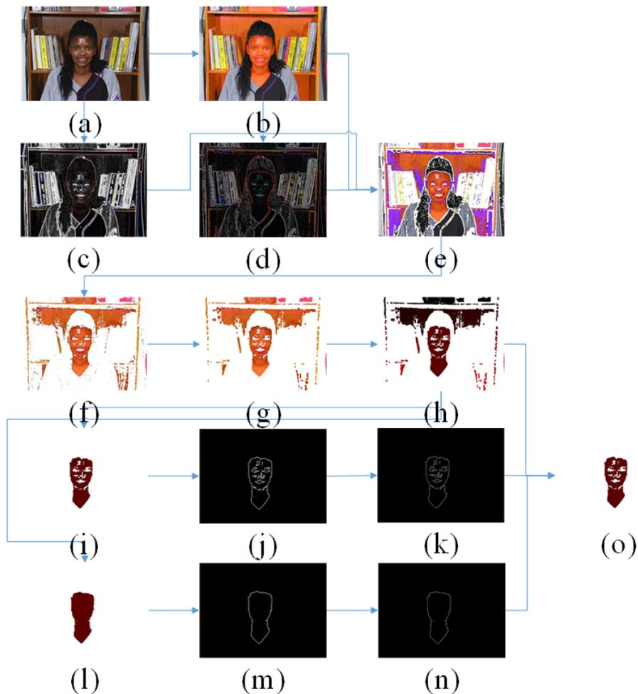
FIGURE 5. The experimental results in a complex background
