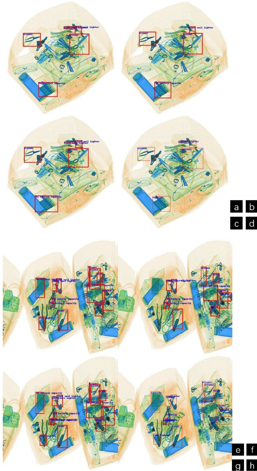
FIGURE 9. Training results of three neural network, an X-ray image with fewer objects (Figure d) is recognized by three neural networks Darknet-19 (Figure a), Resnet-34 (Figure b) and Darknet-53 (Figure c). An X-Ray image with many objects (Figure h) is recognized by three networks Darknet-19 (Figure e), Resnet-34 (Figure f) and Darknet-53 (Figure g)
