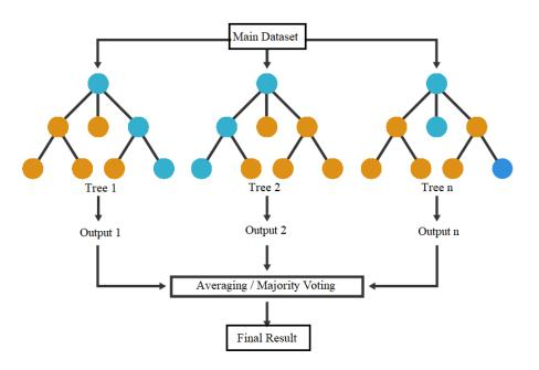
FIGURE 2. Working process of RF classifier in the top-down approach.
