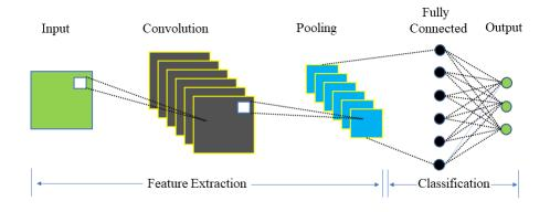
FIGURE 3. Block diagram of CNN
