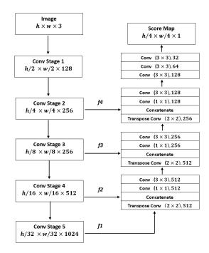
FIGURE 1. The proposed architecture consists of two parts. Feature extraction part (encoder) composed of Darknet53 as backbone and the upsampling part (decoder) which output a prediction map indicating locations of text within the image
