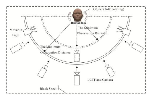
FIGURE 8. Established hyperspectral face imaging system[32]
