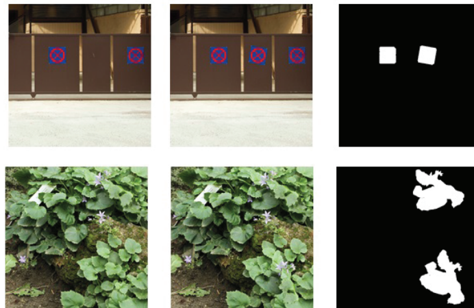
FIGURE 10. Forgery detection for rotated copy-move region. The original images (left), tampered images (middle) and the detected forgery (right)
