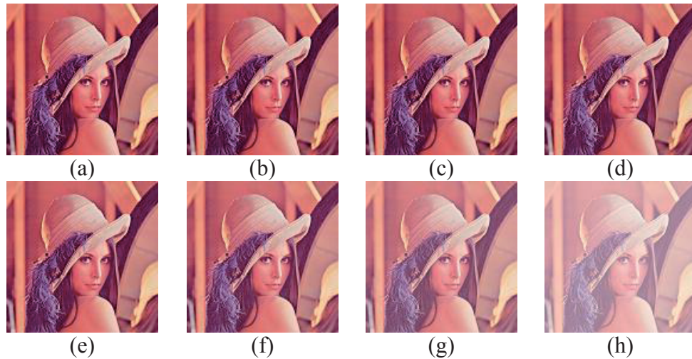
FIGURE 6. PNG image Lena with alpha channel values of (a) 255, (b) 254, (c) 252, (d) 248, (e) 240, (f) 224, (g) 192, and (h) 128.
