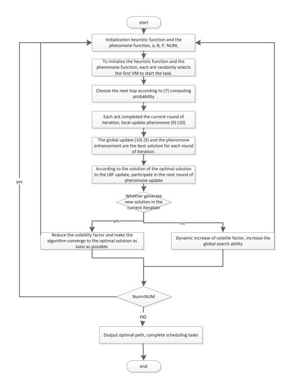
FIGURE 1. The flow chart of the scheduling algorithm
