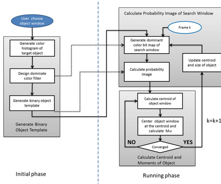
FIGURE 5. The block diagram of the proposed tracking algorithm
