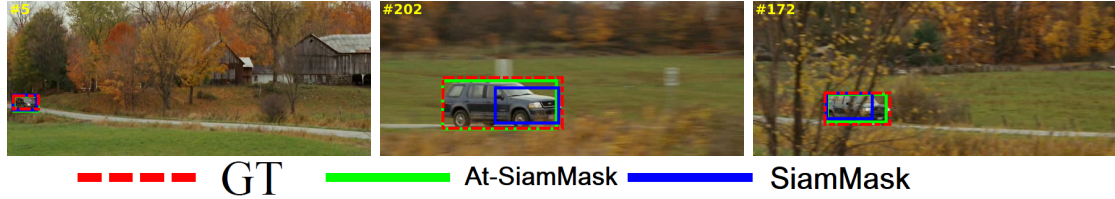
FIGURE 10. Comparisons between SiamMask base tracker and Att-SiamMask on the challenging sequence: CarScale in presence of large scale changes.
