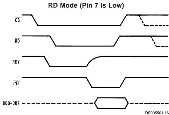
When in RD mode, the comparator phases are internally triggered. At the falling edge of  $\overline{RD}$ , the MS flash converter goes from zero to compare mode and the LS ADC's comparators enter their zero cycle. After 800 ns, data from the MS flash is latched and the LS flash ADC enters compare mode. Following another 800 ns, the lower 4 bits are recovered.
