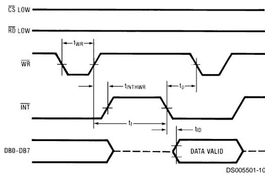
FIGURE 5. WR-RD Mode (Pin 7 is High)
