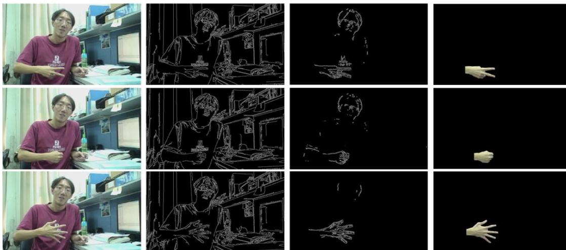
FIGURE 9. HM sequence and its gesture extraction result. The first column shows three frames in nucleus state. The current edge image, the difference edges for gesture, and the extracted gestures are shown in second, third, and fourth column respectively.
