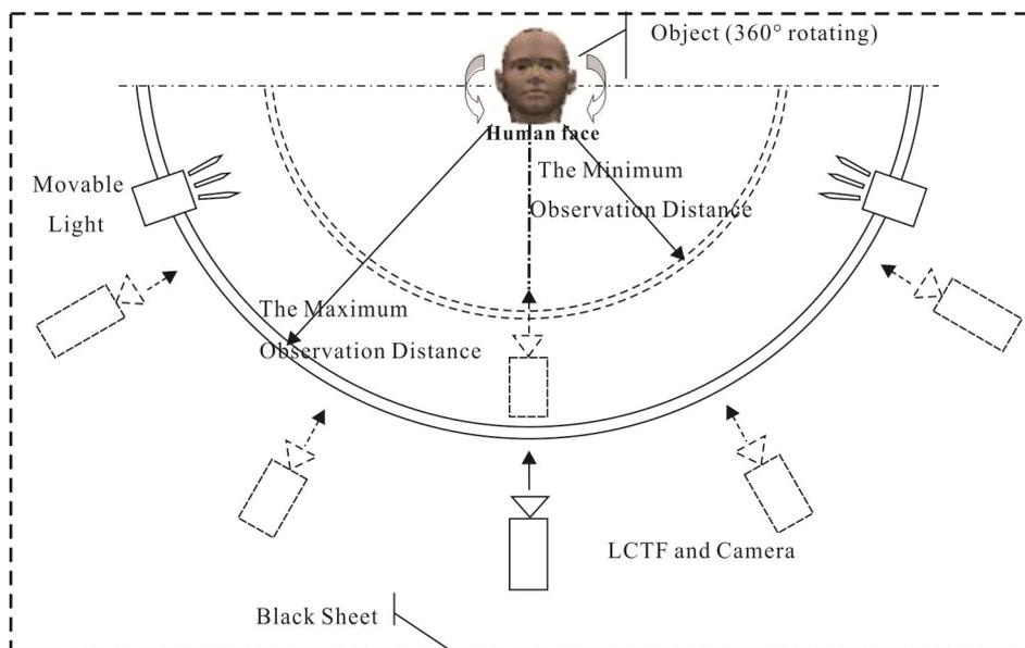
FIGURE 8. Established hyperspectral face imaging system[32]
