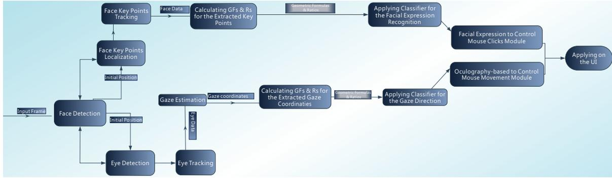
FIGURE 1. Components of The proposed Multi-Modal Oculography-Based Mouse Controlling System : Via Facial Expressions & Eye Movement.
