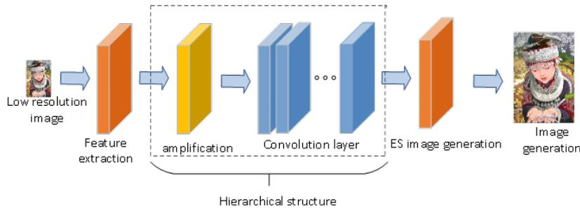
FIGURE 5. The improved generator model.
