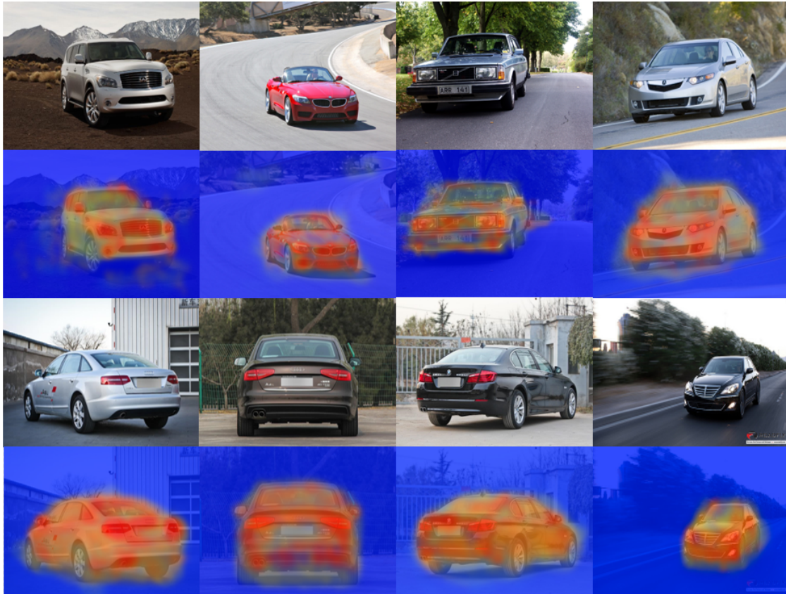
FIGURE 4. Visualization of the discriminative regions. We map each spatial location in the attention map back to the patch in the original image. The results show that the proposed MS-DRAN pays more attention to the discriminative regions of the vehicle.
