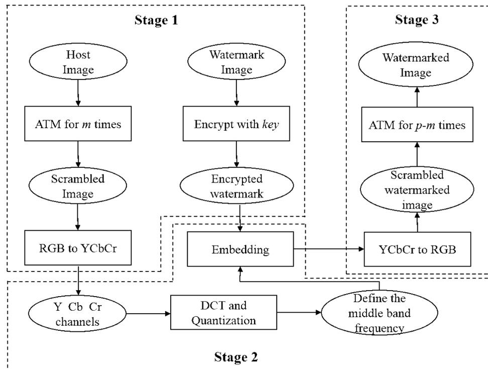
FIGURE 1. The flowchart of the proposed watermark embedding scheme.
